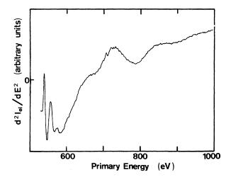
FIG. 2. Second derivative of the elastic yield of the oxidated Al(100) surface, plotted as a function of incident electron energy. The O 1s appearance-potential edge is at 533 eV (correcting for the emitter work function). Fine structure extends several hundred volts above the edge, but the periodic variations are masked considerably by the slowly-varying background.
