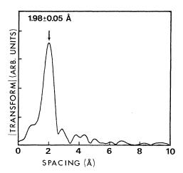
FIG. 4. Optical Fourier transform of the data in Fig. 3, including calculated phase shifts for an O 1s core and Al backscatterers. The single peak at  $R=1.98\pm0.05$  Å is taken as the O-Al spacing in this thin aluminum oxide layer, suggesting that the O lies under rather than over the top layer of Al. See text.
