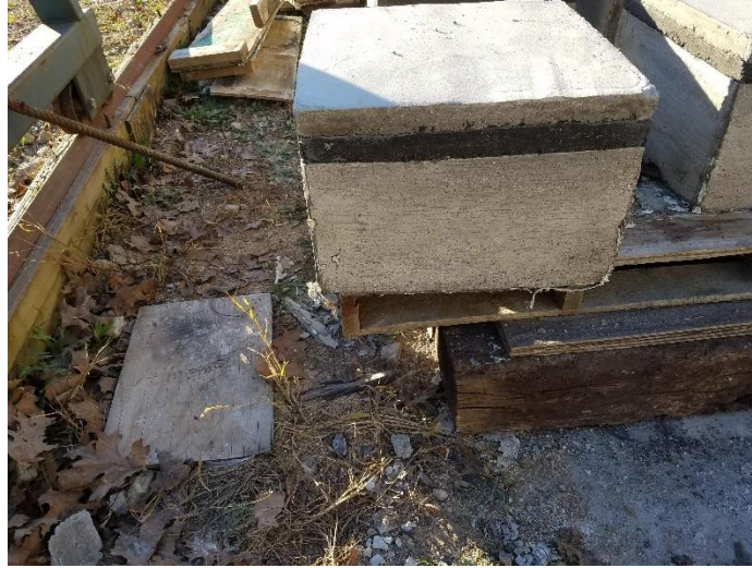
Figure 4.4. Two-Layer Cap Test Specimen
