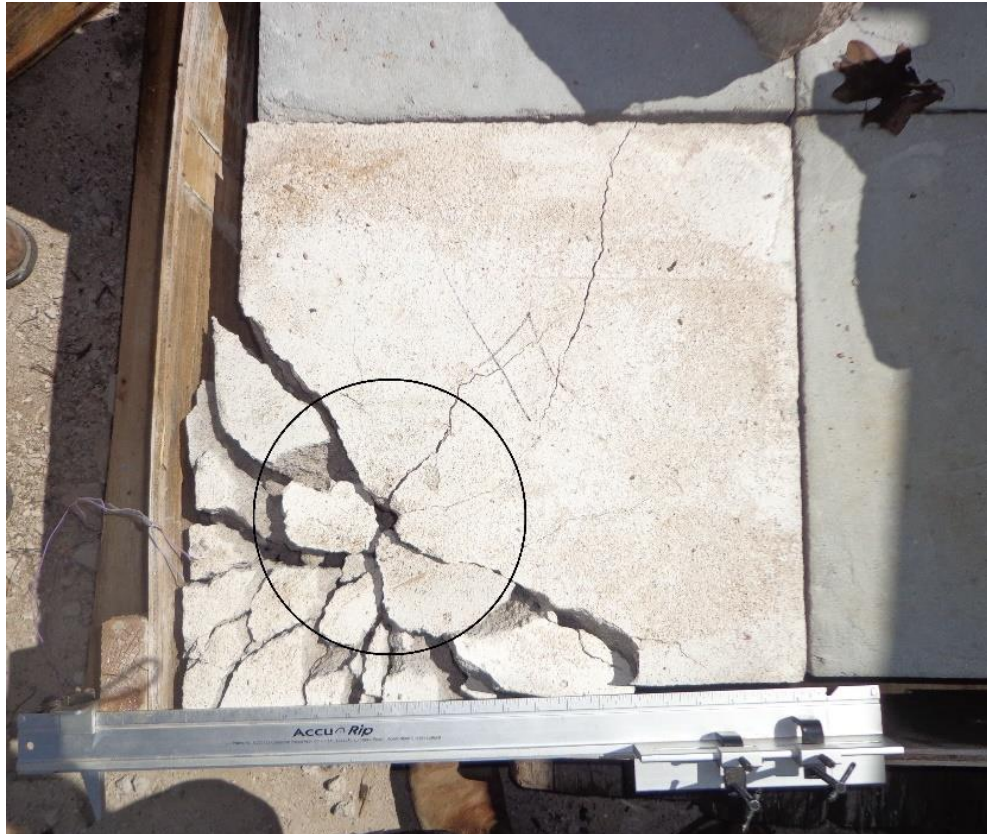
Figure 5.2. Surface Radius of Crater in Solid Block, Test 1 6/7/16
