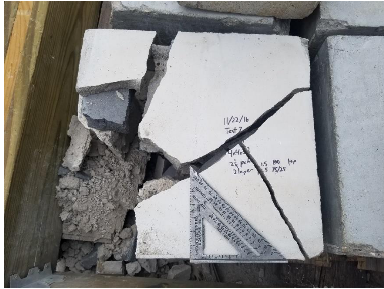
Figure 42 Top Layer Breakage Test 30
