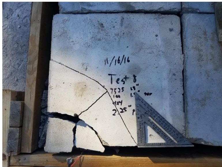
Figure 31 Top Layer Breakage Test 22
