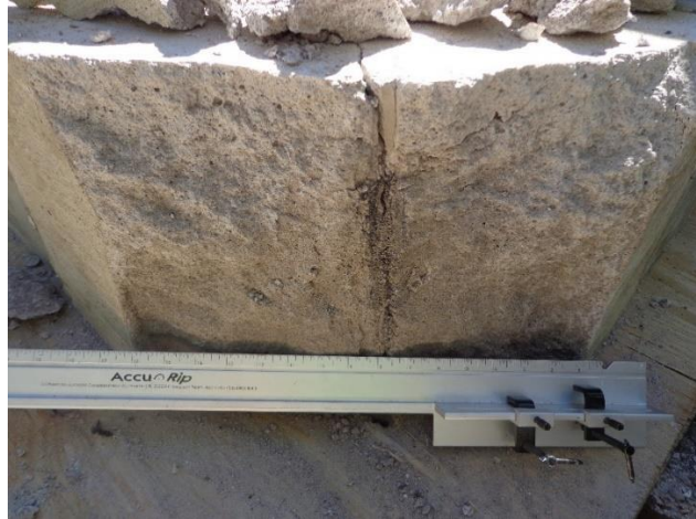
Figure 5.3. Clean-blasted Block Face, Test 1 6/7/16
