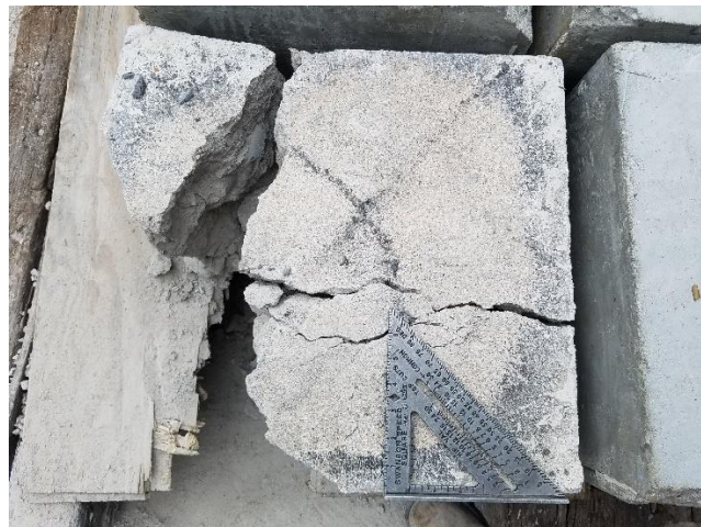
Figure 5.8. Substrate Block Fractures 2-Hole, Test 30 11/22/16
