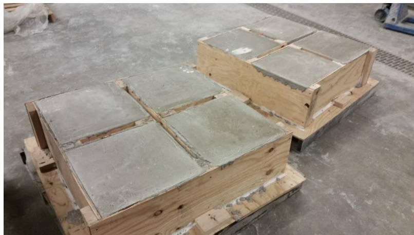
Figure 4.3. Cast Test Specimens in Constructed Forms
