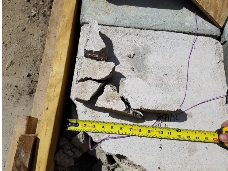
Figure 6.13. Test 13 3" 50%/50% Mix Cap Surface Breakage
