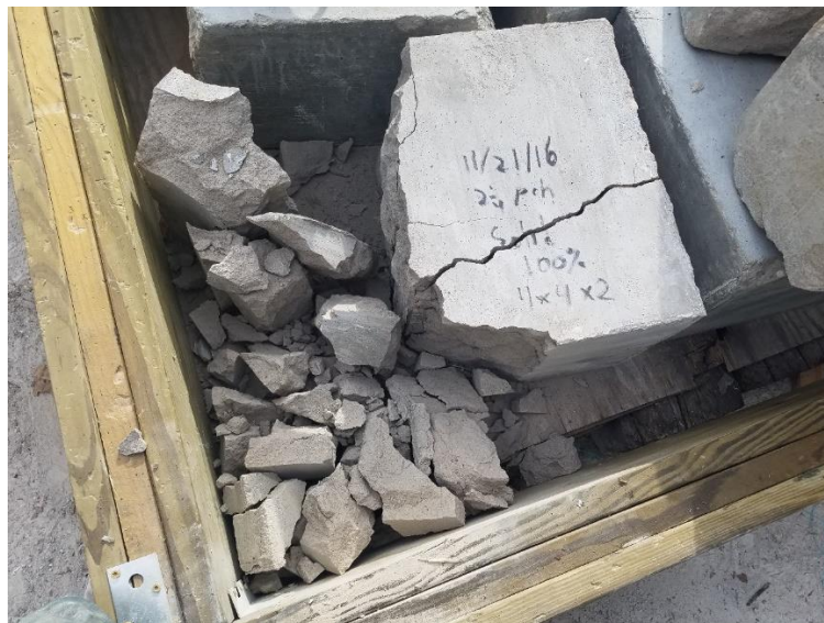
Figure 35 Block Breakage Test 24
