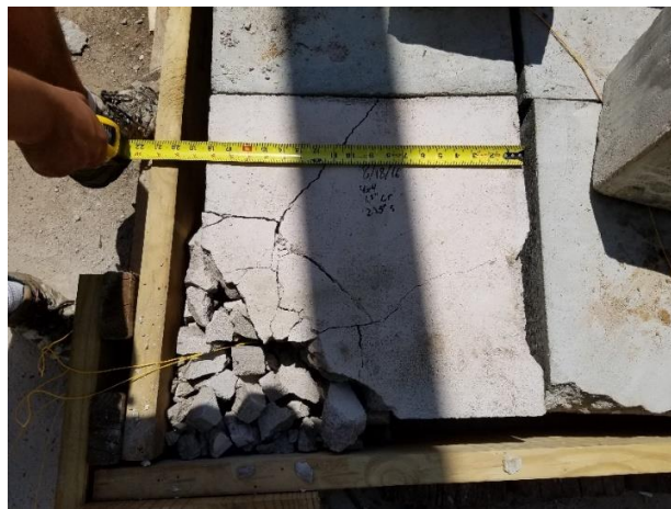
Figure 6.14. Test 9 1.5 in Cap 50%/50% Mix Surface Breakage
