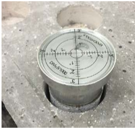
Figure 6-10 High-precision spirit bubble level
