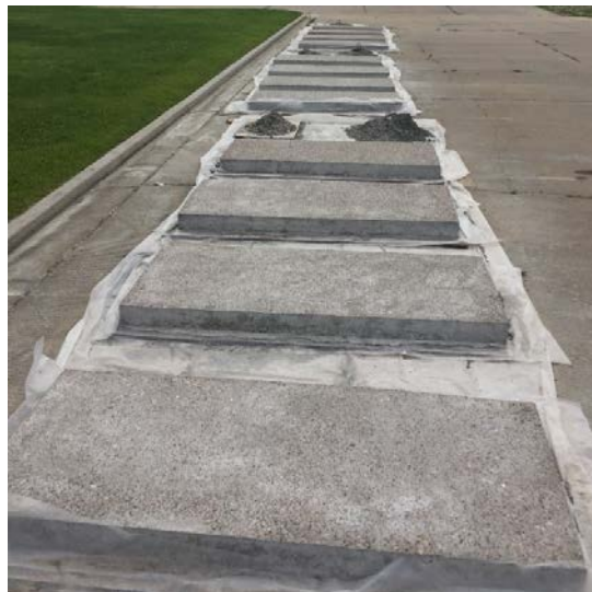
Figure 6-1 Concrete pavement sections as substrate
