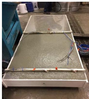
Figure 6-6 Preparation and casting process of UHPC overlay
