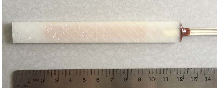
Figure 6-3 Embedded strain gauge for monitoring shrinkage deformation
