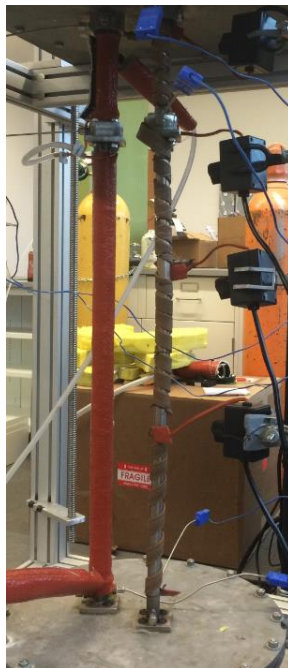
Figure 7. Electrical heaters wrapped around the heated channel
