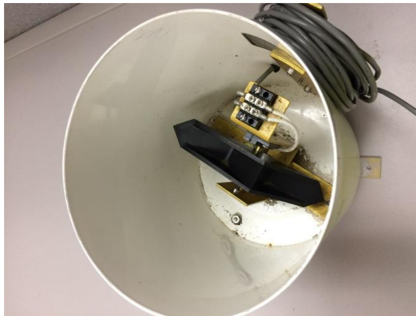
Figure 1.9 Photograph of the tipping-bucket rain gage at the Missouri Department of Natural Resources Groundwater Monitoring Network Well USGS 375625091480401 Ramada Inn Rolla.
