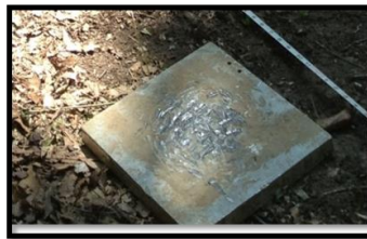
Figure 4.8. The impact steel plate to deliver appropriate impact power into the ground.
