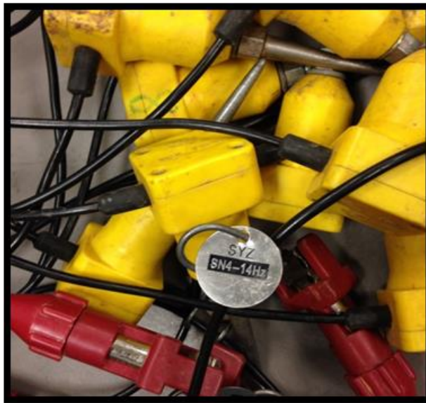
Figure 4.17. A 14 Hz Geophones used for SRT.
