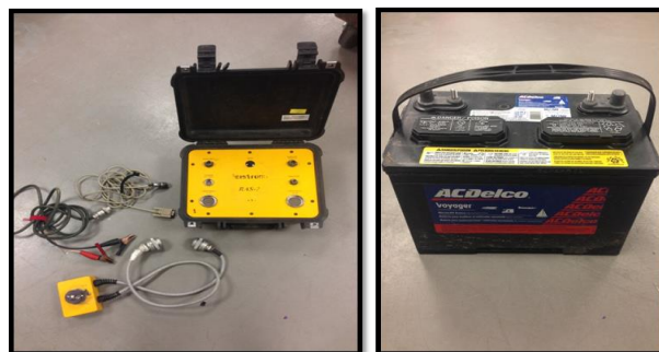
Figure 4.3. The seismograph with its accessories and 12volt battery.
