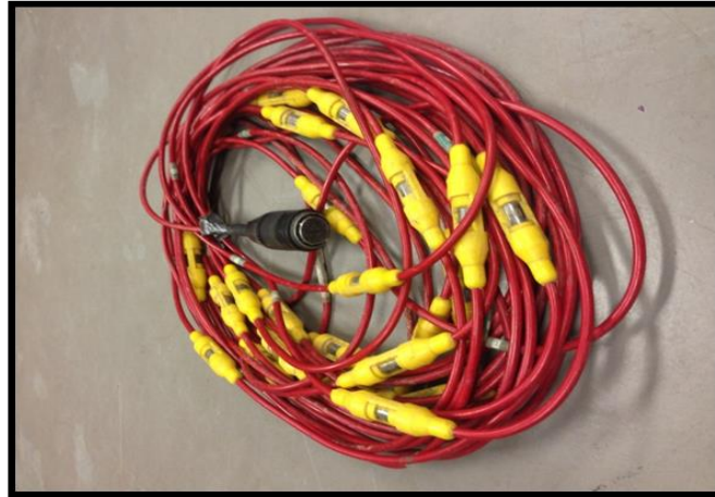
Figure 4.6. Seismic cable with 5ft geophone spacing.
