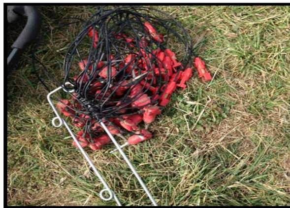
Figure 4.5. A 4.5 Hz Geophone used for MASW.
