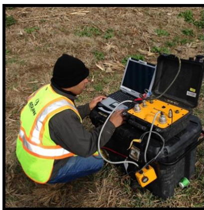
Figure 5.9. Refraction seismic tomography (SRT) acquisition field data.
