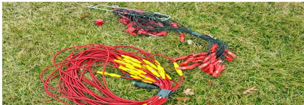
Figure 4.7: Showing cable (red), connectors (yellow), knob (black) and geophones with spike.
