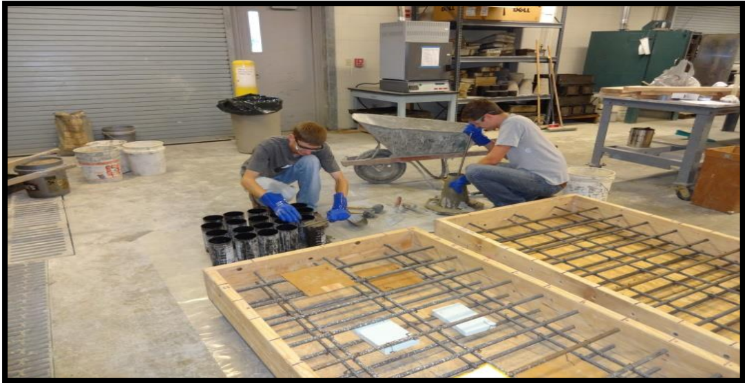
Figure 2.3: Both Slab-2 and Slab-3 before casting
