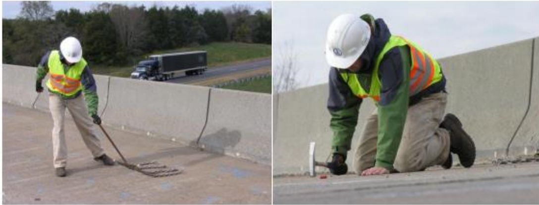
Figure 1.5: Chain drag technique and the hammer technique bridge deck assessment ( www.ndtoolbox.org )
