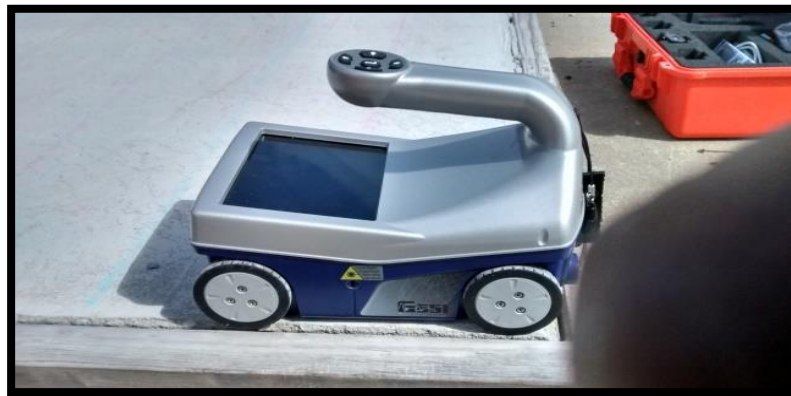
Figure 4.1: Ground Penetration Radar system structure scan mini
