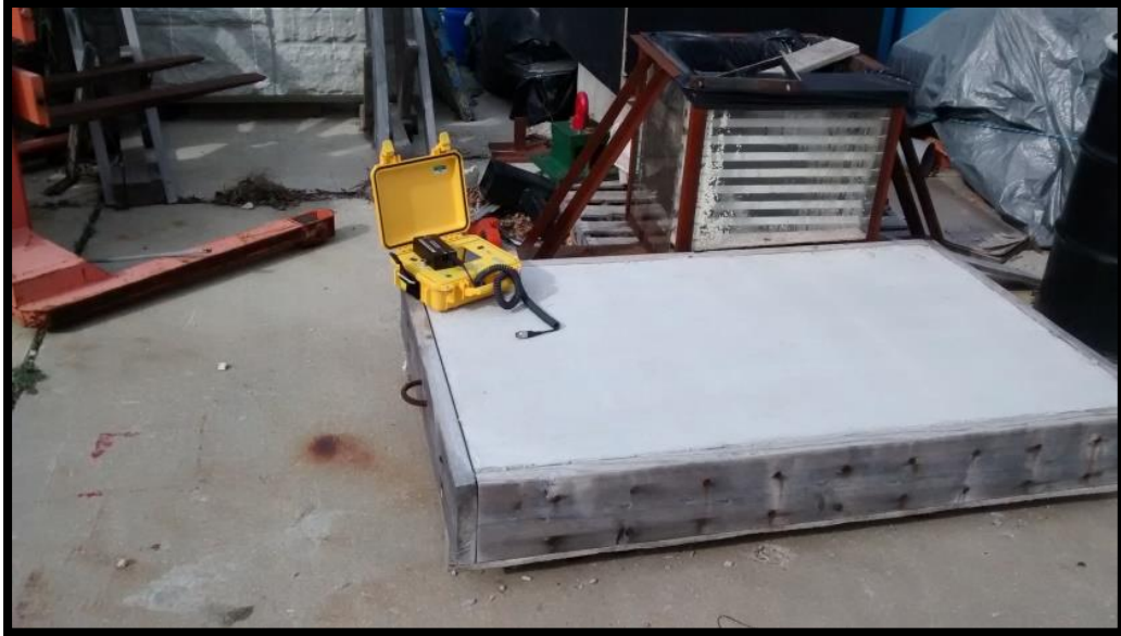
Figure 5.3: Rebarscope data acquisition
