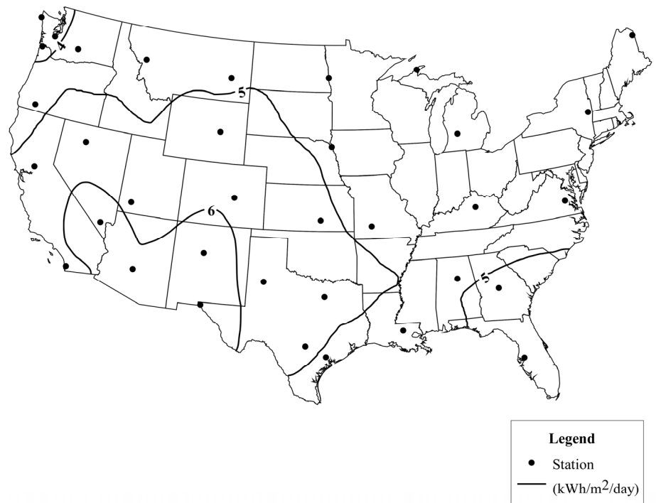
Figure 2. Selected stations and general trend of solar radiation (after NREL 2013).
