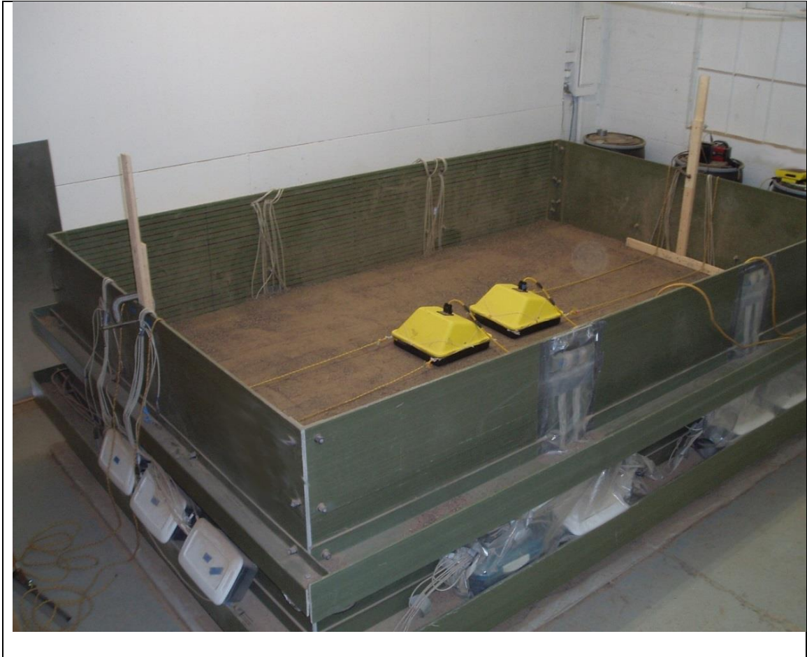
Figure 2.1. The experimental tank was constructed with no metal and filled with flat layers of soil. In this figure, 250 MHz antennas are being moved over dry sand.
