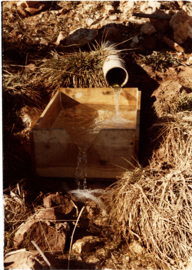
5. Discharge pipe and weir box for blanket drain. Flow estimated at 15 gal/min at time of inspection.
