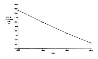
Fig. 3. Cat. reformer design approach temperatures
