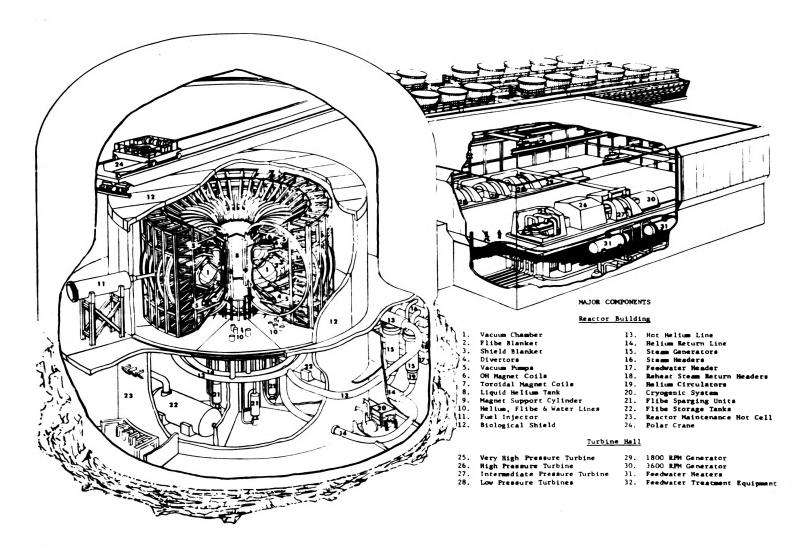
Figure 4-Conceptual design of a tokamak fusion power plant done by the Princeton University Plasma Physics Laboratory, 2,100 megawatts of electricity is produced at 40% efficiency.
