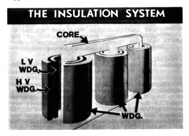
Figure 12. Cutaway view of Transformer
