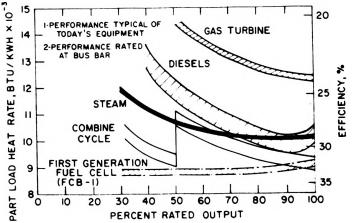
Fig. 4. Energy Systems Comparison .(Part-Load Performance)
