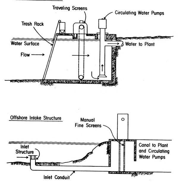
Figure 1. Schematic Diagrams of Typical Intake Structures (Point of Water Inlet to the Water Screening Facility)
