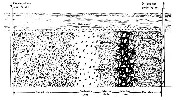
Fig. 5. Schematic diagram of an in situ oil shale retorting process
