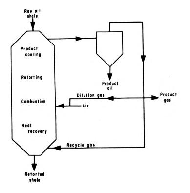
Fig. 4. Gas combustion retort.
