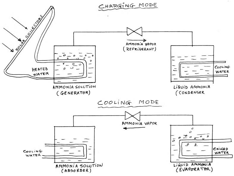
Figure 4. Schematic diagram for a  $\rm NH_3-H_2O$  absorption air-conditioner
