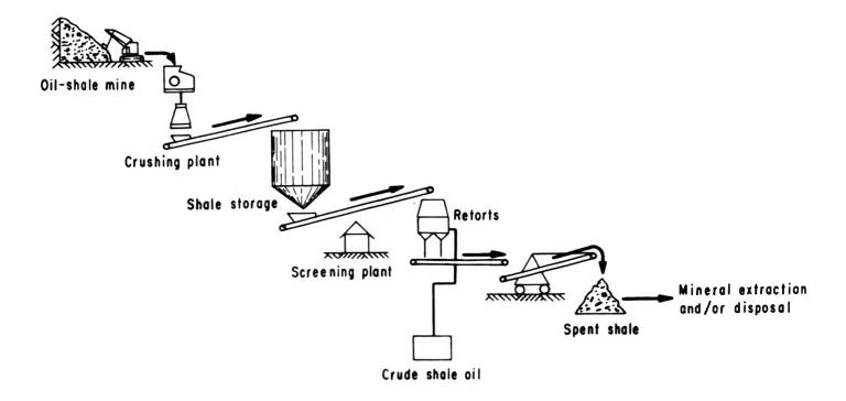
Fig. 3. Schematic diagram of oil shale surface processing.
