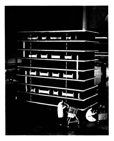
Figure 7. HVDC Conversion System 200 kV Value
