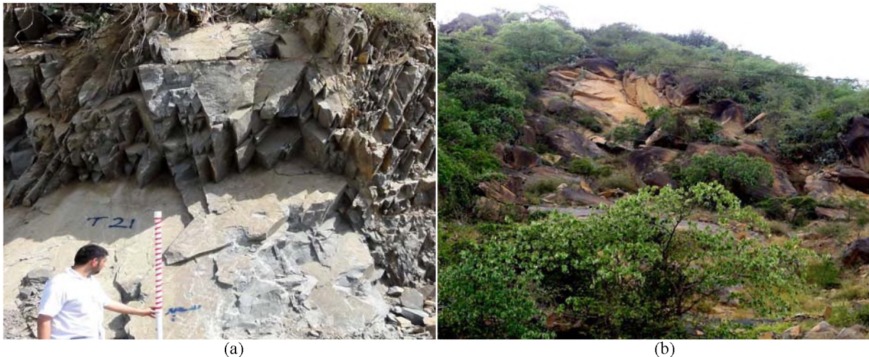
Fig. 8 (a) Rock faces with 100% coverage of natural joint surfaces; (b) rock faces with significant ambiguity as to the location of natural joint surfaces.
