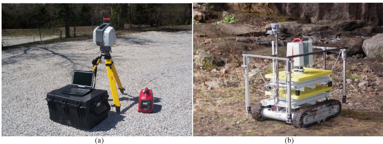
Fig. 7 (a) Leica ScanStation II time of flight scanner with integrated optical camera; (b) Leica HDS 6000 phase shift scanner on remote controlled robotic buggy.
