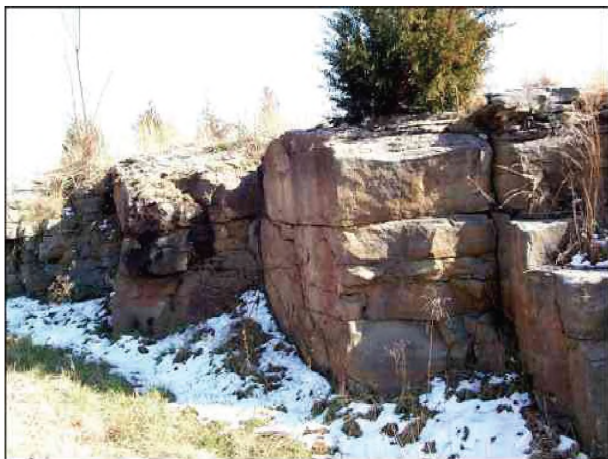
Fig. 2 Orthogonal nature of joint sets. Measurements of the “cracks” or discontinuities are displayed in Fig. 3.
