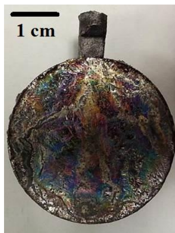
Figure 2.11. An immersion sample taken from the melt.
