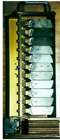
Figure 2.12. Vertically focusing Ge wafer monochromator at HRPT[32] .
