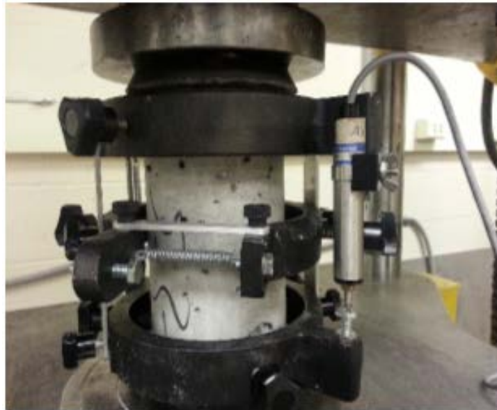
Figure 5.2 Modulus of elasticity test setup
