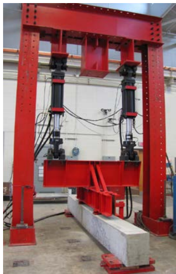
a) Test set up and load pattern
