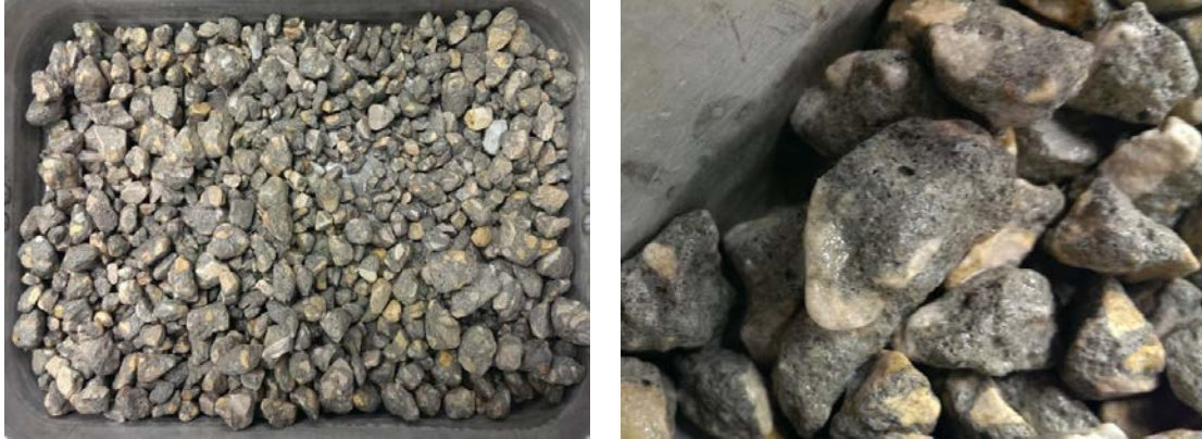
Figure 3.2 Laboratory produced coarse RCA
