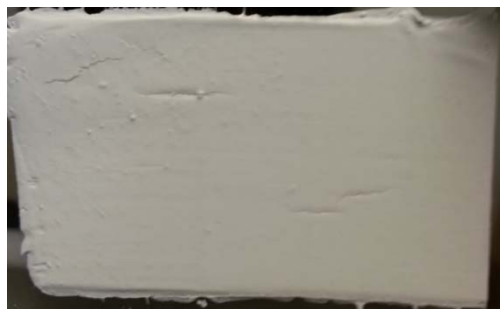
Figure 5. Cracks as a result of fast drying.
