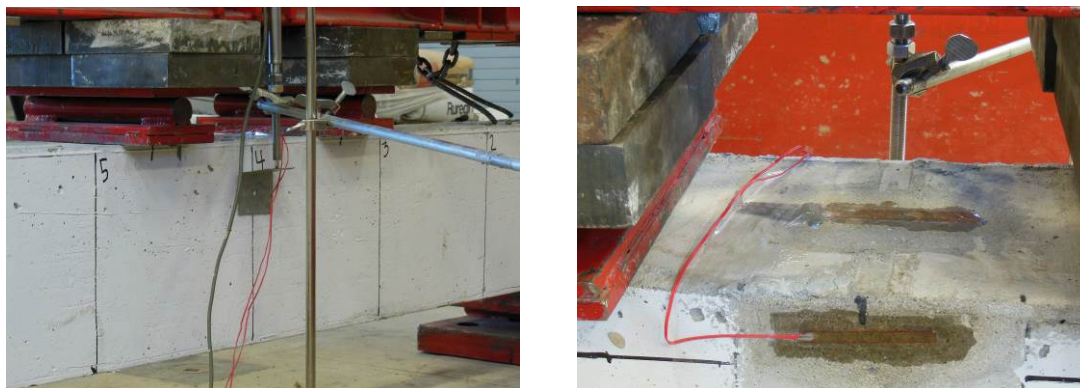
Figure 9-14 Installation of LVDT (left) and strain gauges on surface of concrete beam (right).
