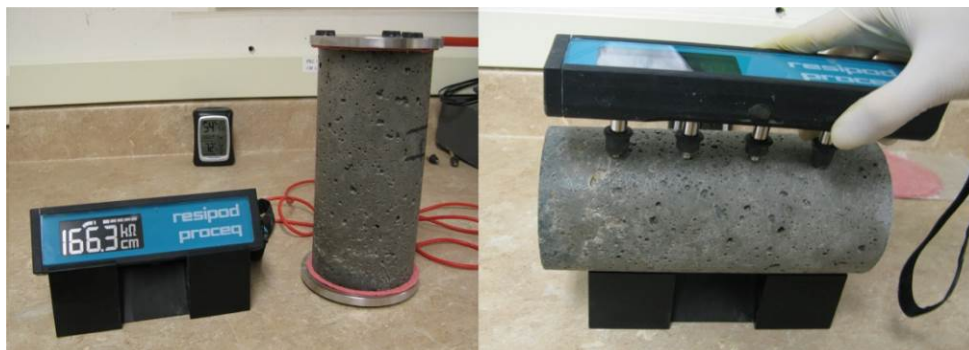
Figure 8-7 Bulk electrical conductivity (left) and surface resistivity (right).
