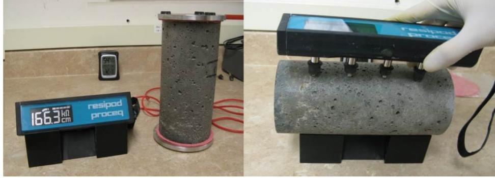
Figure 3-7 Bulk electrical conductivity (left) and surface resistivity (right).
