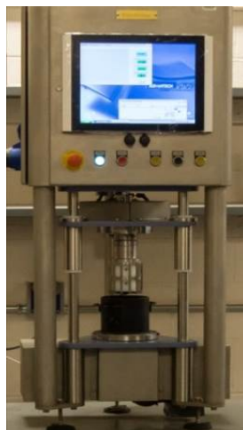
Figure 3-5 Coaxial cylinders rheometer.
