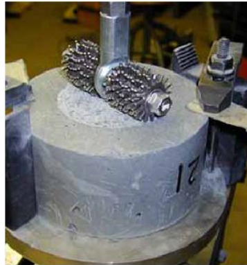
Figure 8-5 Abrasion resistance test setup.
