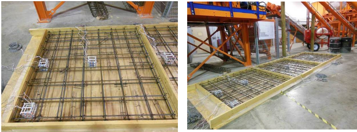
Figure 9-1 Slab section used for shrinkage deformation evaluation.
