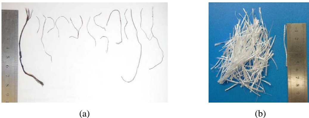
Figure 8-2 Fiber types used in this study: (a) recycled steel fibers and (b) synthetic fibers.
