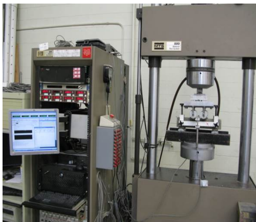
Figure 8-4 Test setup for flexural toughness measurement of FRC beams.
