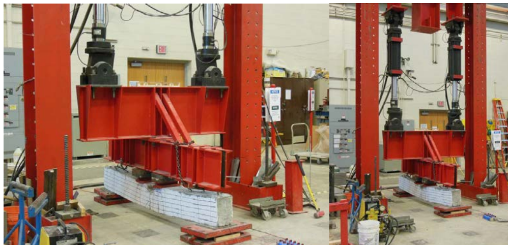
Figure 9-12 Beam flexural test setup.
