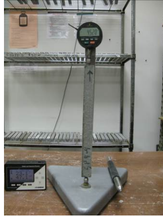
Figure 3-6 Drying shrinkage measurement.
