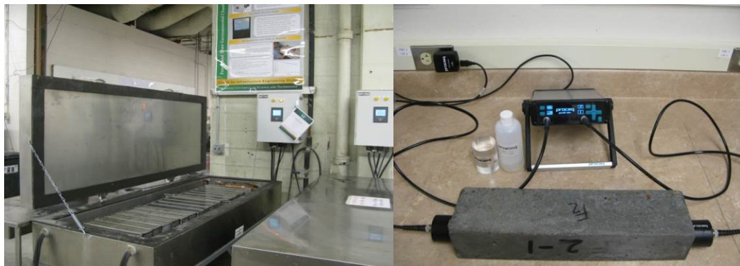
Figure 8-6 Freeze-thaw chamber (left) and ultrasonic velocity instrument (right).
