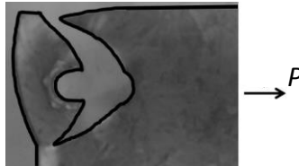
Figure 3 Localised tearing (extracted from Casafont et al. (2006))
