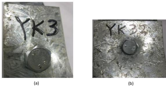
Figure 4 Two orientations of bolt head and nut: (a) Orientation I; (b) Orientation II
