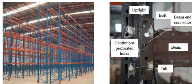
Figure 1. Pallet racks and typical beam-to-upright bolted connections
