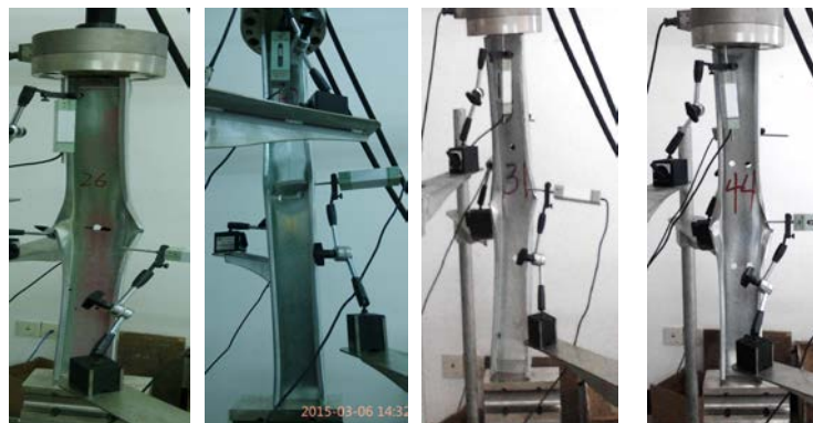
(a) One hole in one row (b) Two holes in one row (c) Two holes in one column (d) Four holes in two rows and two columns
