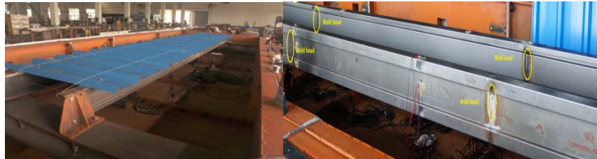
Figure 17: Overall test assemblies Figure 18: The purlin with weld beads
