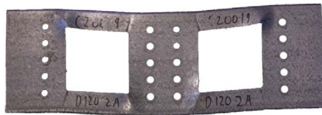
Fig. 7. Failure mode on shear test on C20019-S120 member
