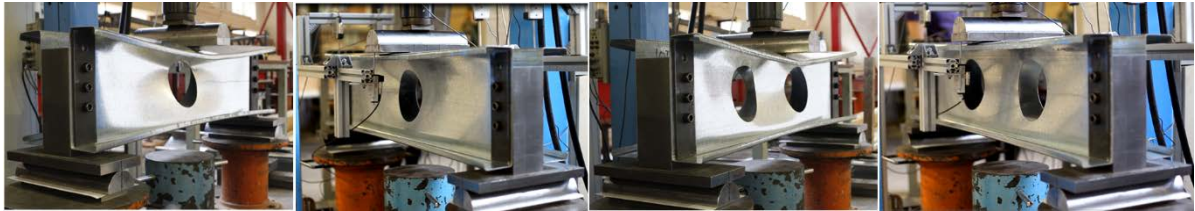
Figure 1: Experimental analysis of cold-formed steel channel sections under IOF loading condition
