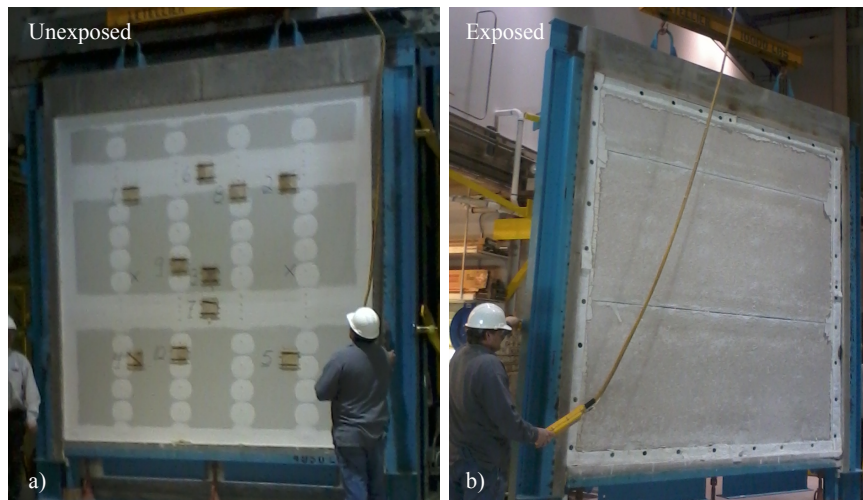
Figure 14: CFS wall after standard fire test, a) unexposed and b) exposed boards
