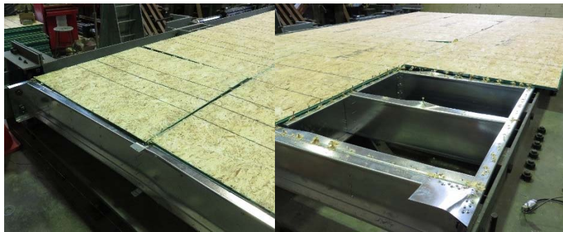
Figure 9 – Test 12-RSTRAP-M sheathing connection failures (left) and Test 13-FB4-M sheathing connection failures with compression field damage to steel frame (OSB panel removed for photograph) (right)
