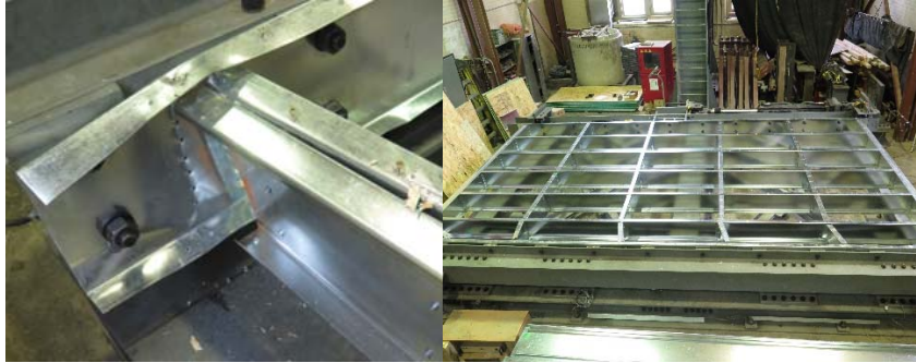
Figure 8 – Test 11-RALT-M failure of chord to rim joist connection (left) and hinge created in the CFS frame after loss of the sheathing connections (right)
