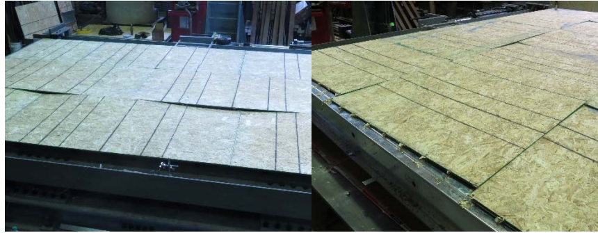
Figure 10 – Test 14-RGY-P-M OSB panel lift-off (left) and Test 15-RGY-P-C sheathing connection failures (right)
