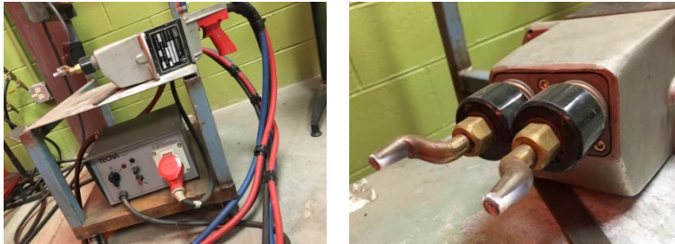
Figure 4 - Spot-welding machine and “A” pointed double bent shanks
