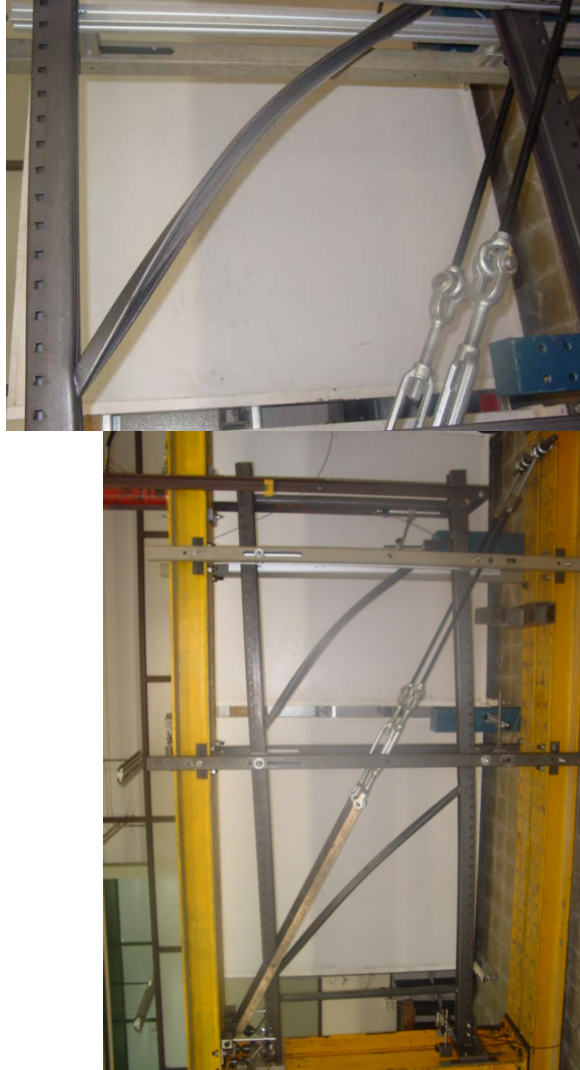
Fig. 8 Frame type A column Test Set-up – Diagonal in compression
