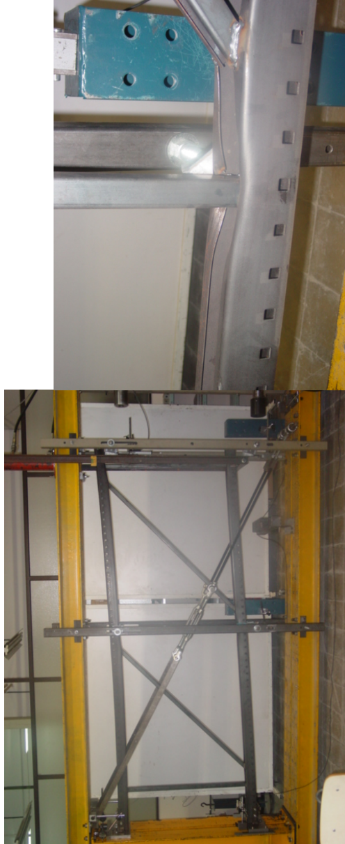
Fig. 6 Frame type A column test set-up - diagonal in tension
