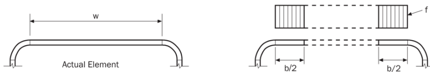
Figure 4 – Flange Under Compressive Stress, Effective Element Width, b
