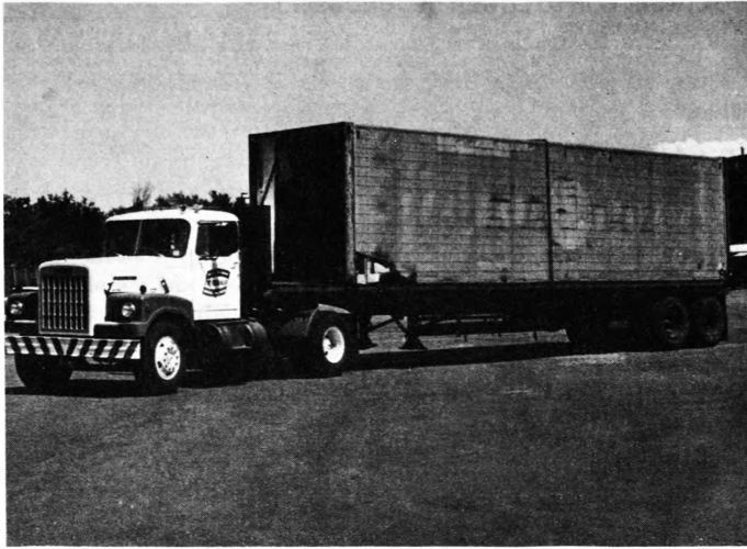
Fig. 1. Dry Freight Container (35-foot)
