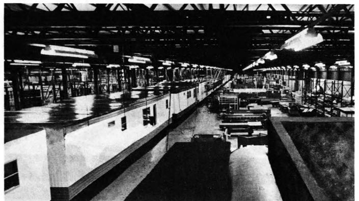
Fig. 15. Main Assembly Line (End-by-End Type): Window/Door Installation (Richardson Homes Corp., Elkhart, Ind.)
