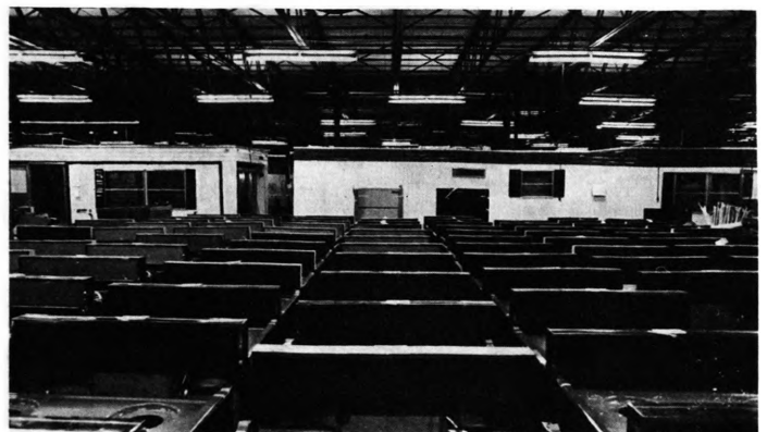
Fig. 16. Main Assembly Line (End-by-End Type): Appliance Feeding (Richardson Homes Corp., Elkhart, Ind.)
