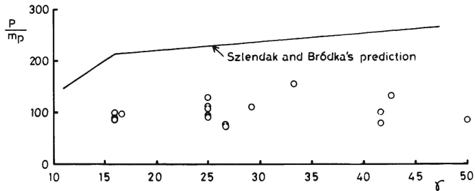
FIG.9.-COMPARISON OF TEST RESULTS AND SZLENDAK AND BRÓDKA'S PREDICTION
