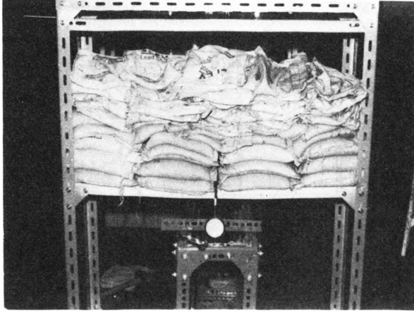
FIG 3 MEASURING DEFLECTIONS UNDER LOAD
