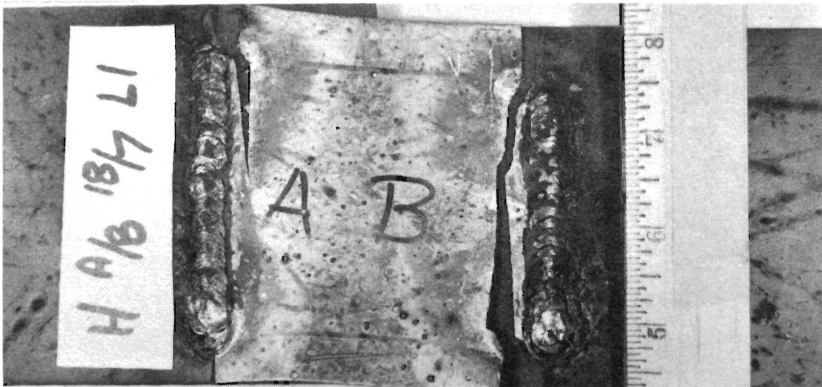
Sheet Tear Transverse Fillet Weld
