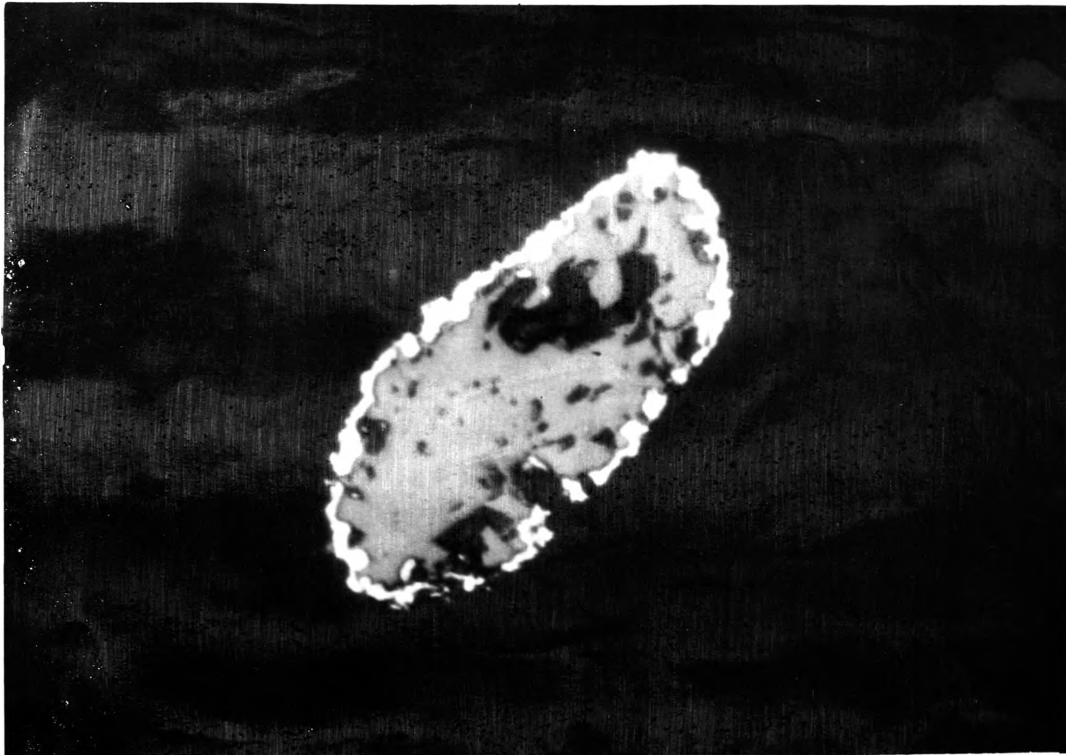
Figure 9. Coal particle coated completely with metallic lead. Magnification: 550x
