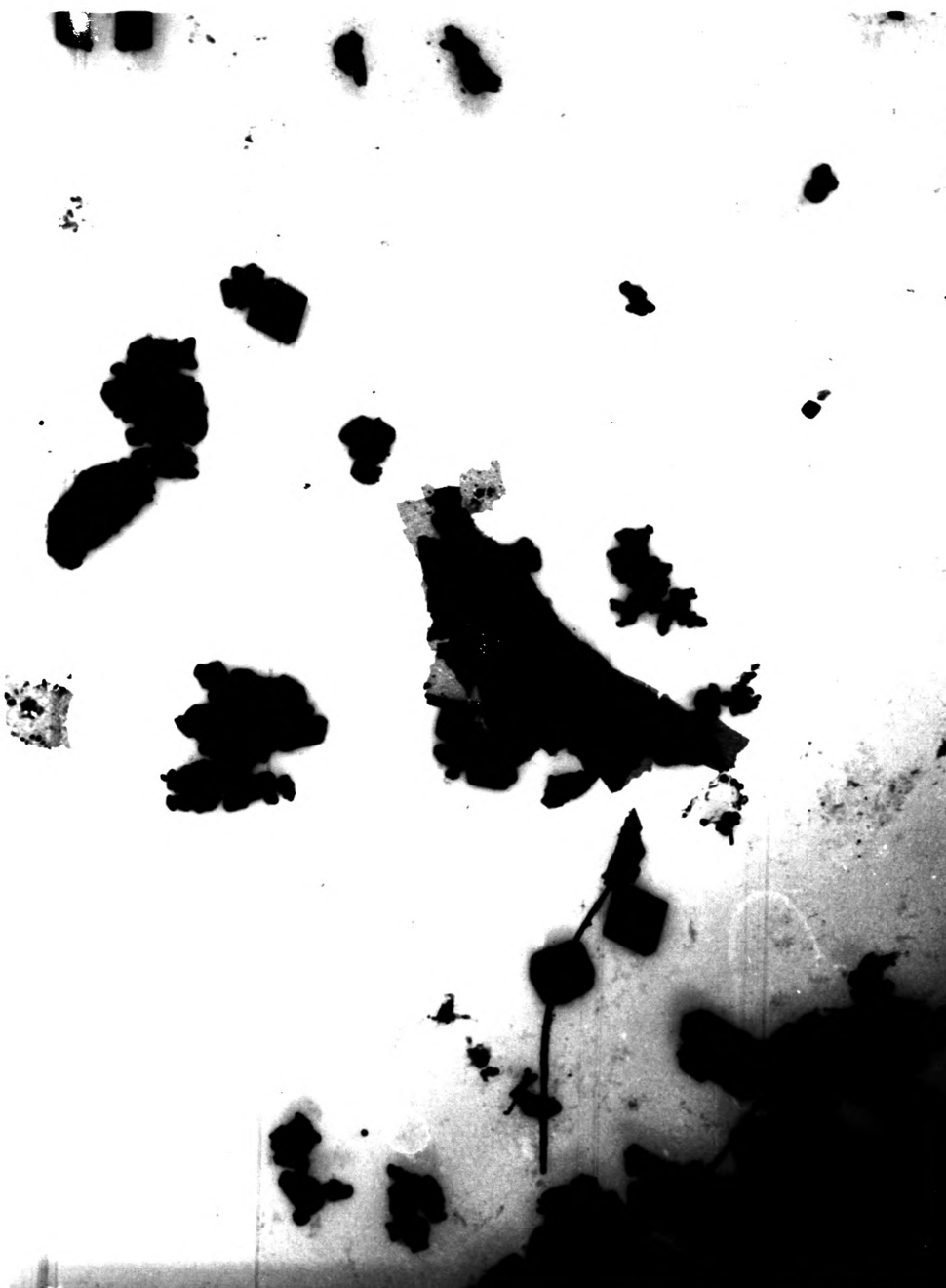
Figure 3. Electron micrograph showing copper particles with typical dendritic or skeletal shapes as a result of rapid crystal growth Total magnification: 4,375 Dispersion: None Shadowing : None
