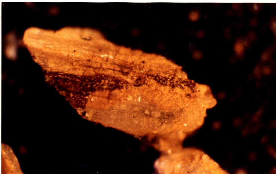
Figure 5. Particles of cerussite coated with various thin layers of limonite (yellowish and brownish colors). The cerussite has a transparent glassy to whitish appearance. Limonite specks pepper over the free surface of the cerussite. Mesh size: 80 to 100
