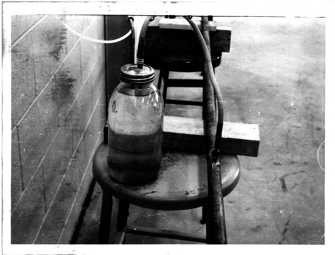
Figure 6, Manometer Connection and Sand Trap
