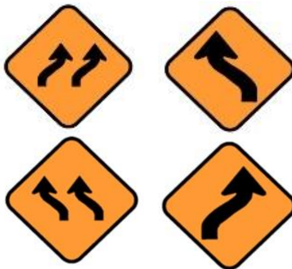
Figure 4.1. MUTCD lane shift sign configuration
