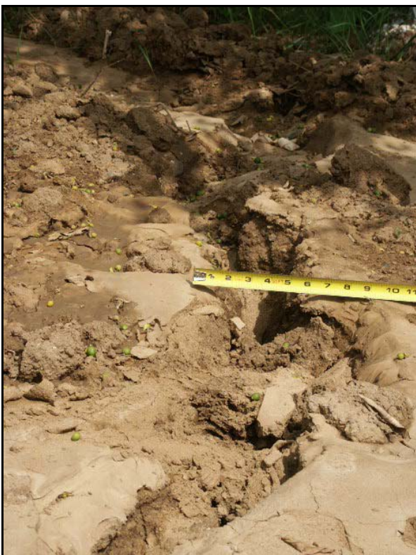
Fig. 15. Liquefaction-induced sand boils and sand vent in an orange grove in Zemmouri
