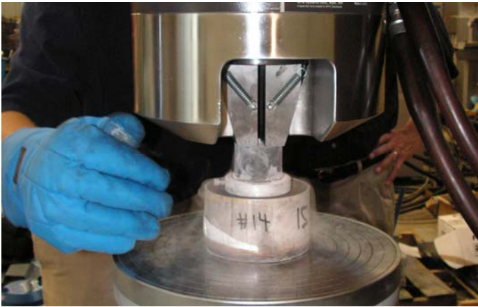
Fig. 4. A sample ready for indentation.
