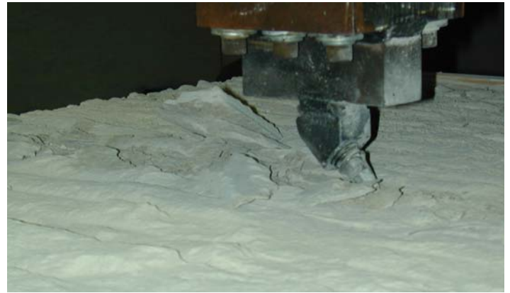
Fig. 18. Linear cutting test of a conical bit in Salem Limestone.
