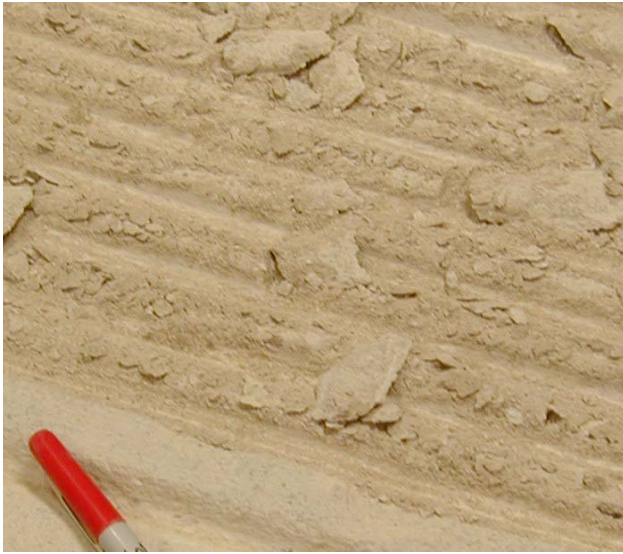
Fig. 20. Typical fragmentation when critical penetration has not been reached. S/P ratio is 10.
