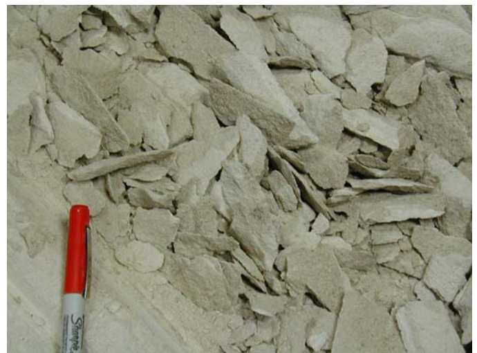
Fig. 19. Typical fragmentation when critical penetration is reached. S/P ratio is 3.3.
