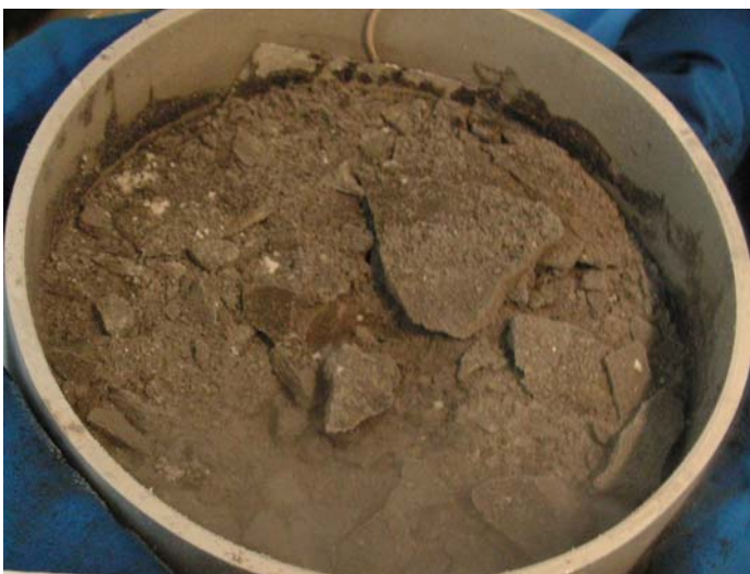
Fig. 8. The brittle, energetic failure pattern typical of saturated samples.
