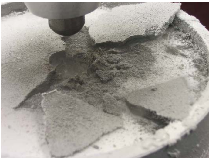
Fig. 5. Close view of a sample immediately after indentation, showing some of the chips and the fines produced.
