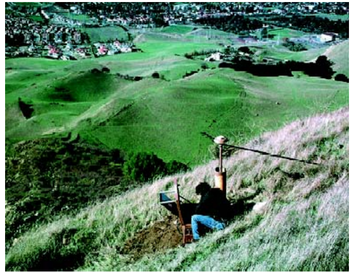
Fig. 7. The lower station was located on the moving block. Both GPS and radio antennas are on the mast near the electronics package inside a box with a 20 watt solar panel.
