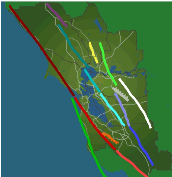
Fig. 25. Earthquake fault source map displayed on ABAG's web site. The active fault segments are color-coded and listed on a table.
