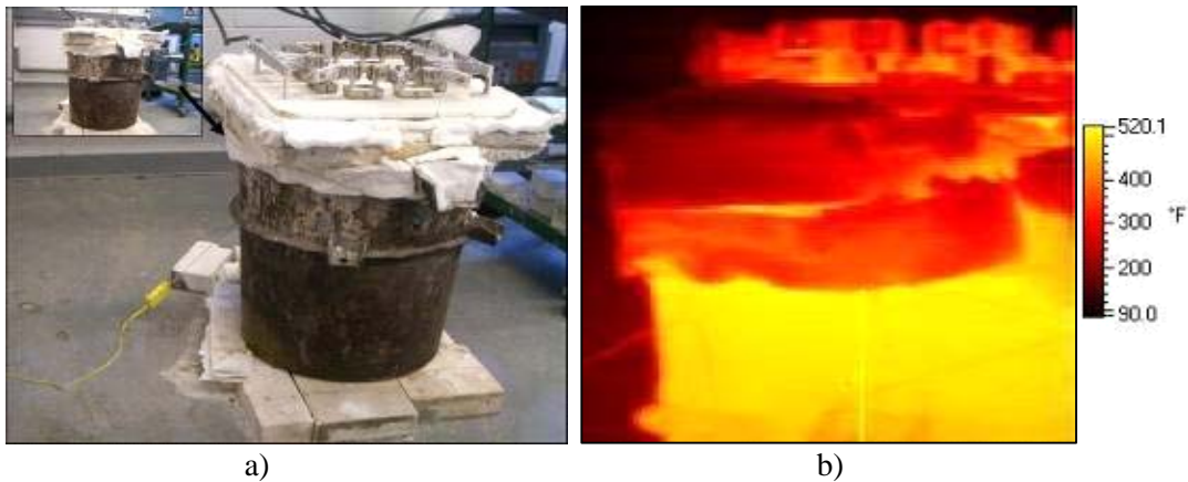
Figure 12. (a) Ladle during initial soaking and (b) steel shell temperatures during the soaking process.
