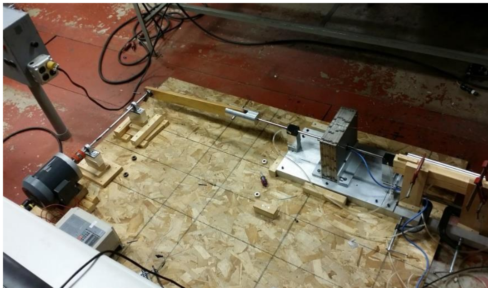
Figure 6.9: Linear Generator coupled with Mechanical system
