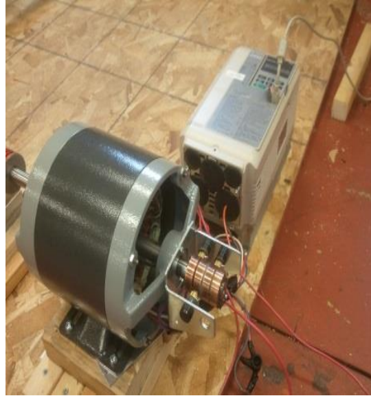
Figure 6.5: Motor with VFD
