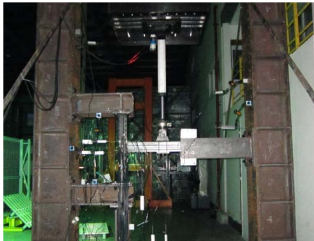
Figure 7 Cantilever test specimen and set-up
