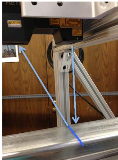
Figure 3 Detail of line laser measurement of the web of a specimen
