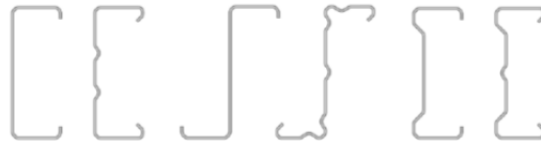
Fig. 1. Conventional CFS profiles with or without stiffeners
