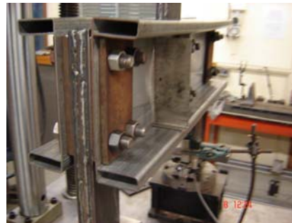
Figure 5: Web with Two Full WSP for 200x45x1.6 LSB
