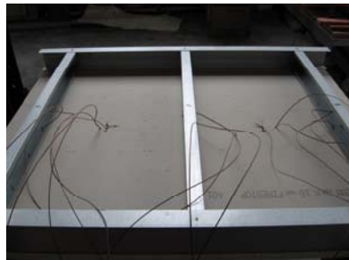
Figure 3: Installation of K type wire thermocouples in Test Specimens
