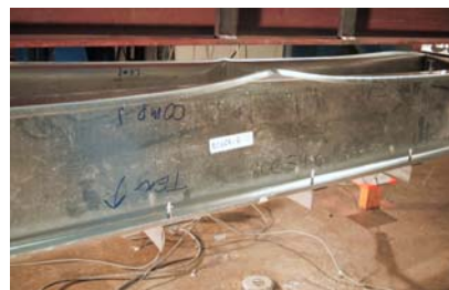
(b) unrestrained 800S200-054 C exhibiting distortional buckling
