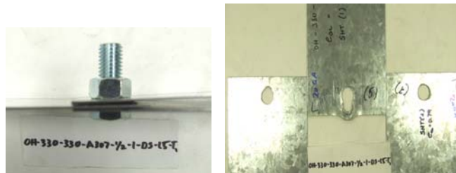
Figure 7 Failure mode of double shear connection OH-330-330-A307-1/2-1-DS-1.5-T1
