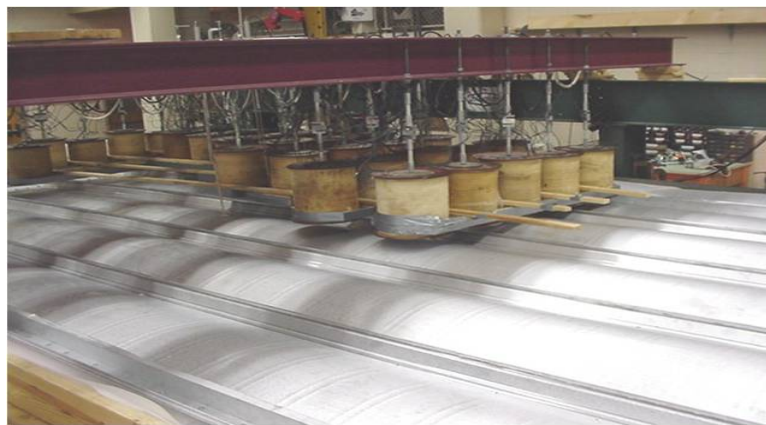
Fig 5. Electromagnetic uplift Testing - Back View
