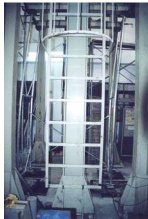
Fig. 6 Test result of scaffolds with removal of cross-brace at access location under concentric loading
