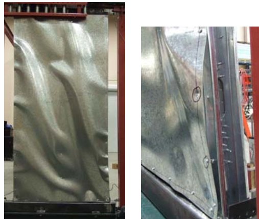
Figure 7 Failure modes for test 4x8x43x33-6/12-M1
