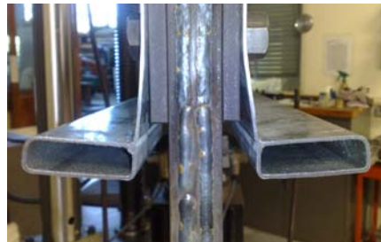
Figure 6: Web with by One Full WSP for 200x45x1.6 LSB
