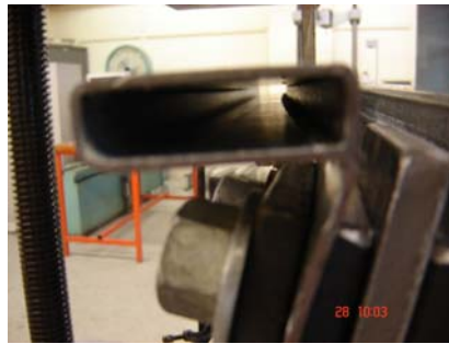
Figure 4: Web with Two Partial WSP for 200x45x1.6 LSB
