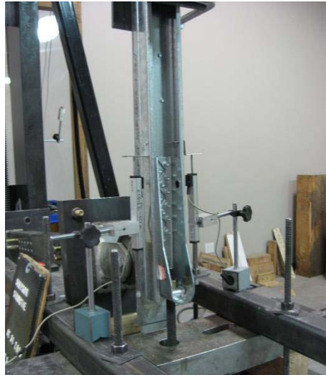
Figure 6 – Raised hold-down Assembly Tension Test Setup – Front
