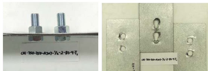
Figure 12 Failure mode of double shear connection OH-300-300-A307-1/2-1-DS-4-T1
