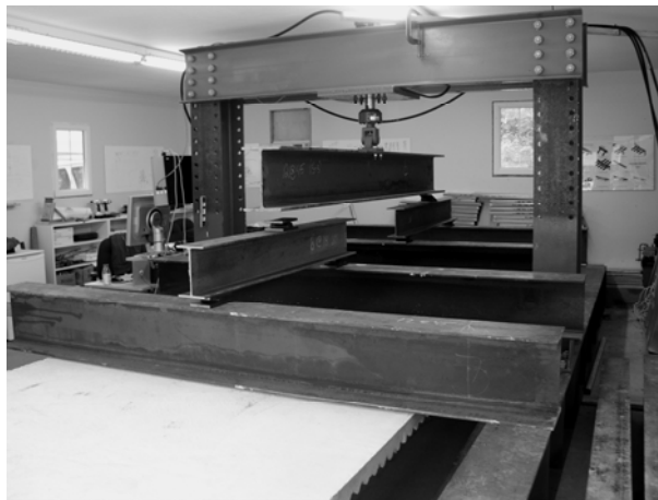
Figure 4 - Photograph of Full Scale Flexural Test Setup
