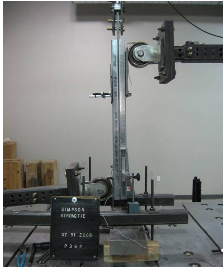
Figure 5 – Raised hold-down Assembly Tension Test Setup – Side
