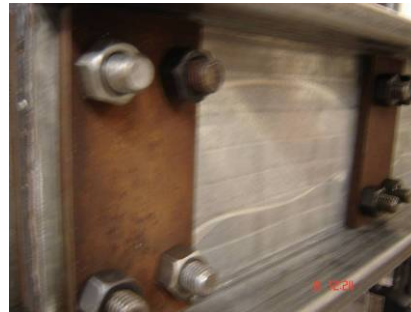
Figure 9: Inelastic Shear Buckling 200x60x2 LSB
