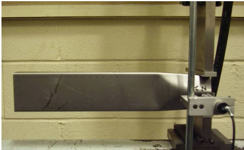
Figure 6: Photograph showing ETF loading test rig with displacement transducer.
