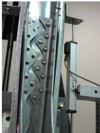
Figure 7 - Hold-down Assembly Tension Test Failure – Screw Shear
