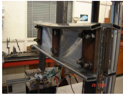
Figure 8: Elastic Shear Buckling 200x45x1.6 LSB
