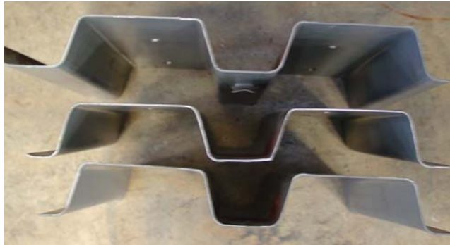
Figure 10. Deformation of Deck Type B1 and B2
