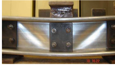
Figure 7: Shear Yielding Failure (125x45x2 LSB)
