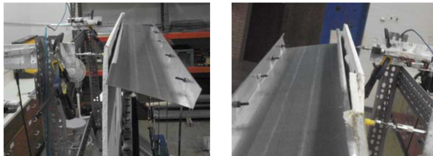
(a) large separation between joist and gypsum board
