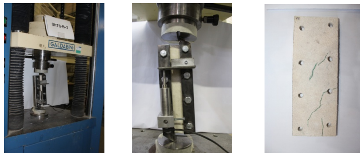
Figure 11: Test set-up for edgewise shear test and failure mode.
