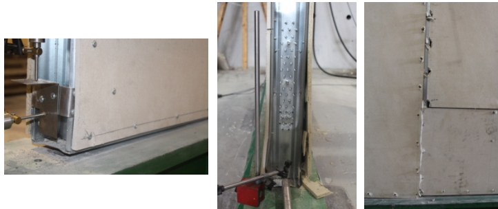
Figure 9: Failure mode for wall G8.
