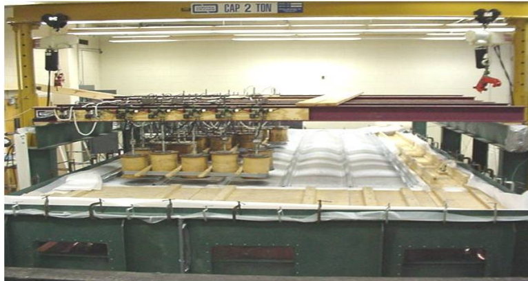
Fig 4. Electromagnetic uplift Testing - Front View of 34 Nodal Points Placed as per UWO Area Distribution
