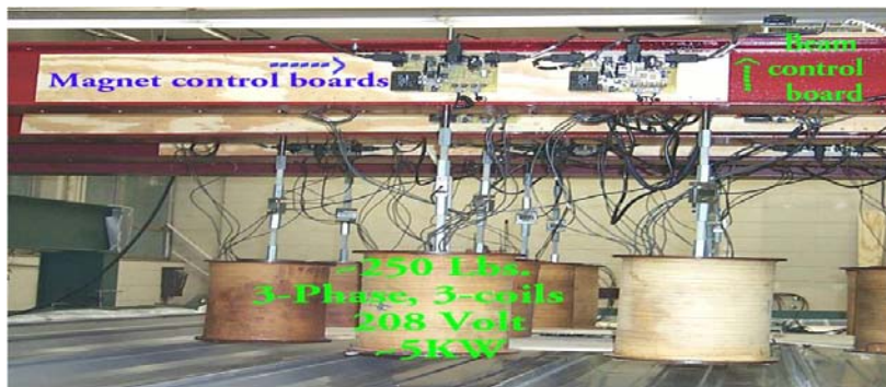
Fig 3. Electromagnetic uplift Testing - Group of Electromagnetic Nodal Points
