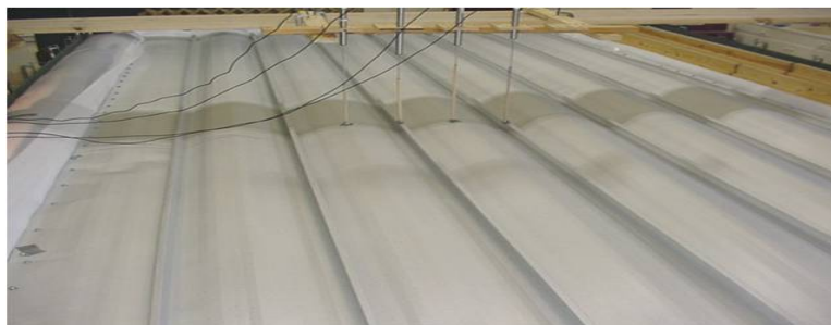
Fig 10. Uniform Static Pressure Tests- ASTM E-1592. Houston Vertical Legs Roofs – During Loading.
