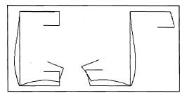
Figure 4 Flange-lip distortional buckling mode
