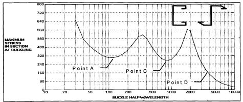
Figure 1 Buckling stress vs Half-wavelength for sections with shallow lip stiffeners
