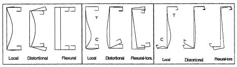
Figure 2(a) Channel in Compression Figure 2(b) Channel in Flexure Figure 2(c) Z-section in Flexure
