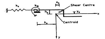
Figure 5 Flange-lip combination elastically restrained along flange-web junction
